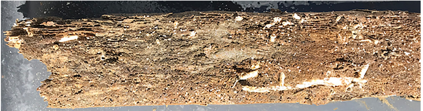
Fig 11. Wooden post from eulittoral test rack. Post from untreated larch wood after 26 months of exposure at the Mediterranean test site. The wood is perforated by wood-boring bivalves (white tubes) and broken. Scale: white tube lower right is about 5 mm diameter.
