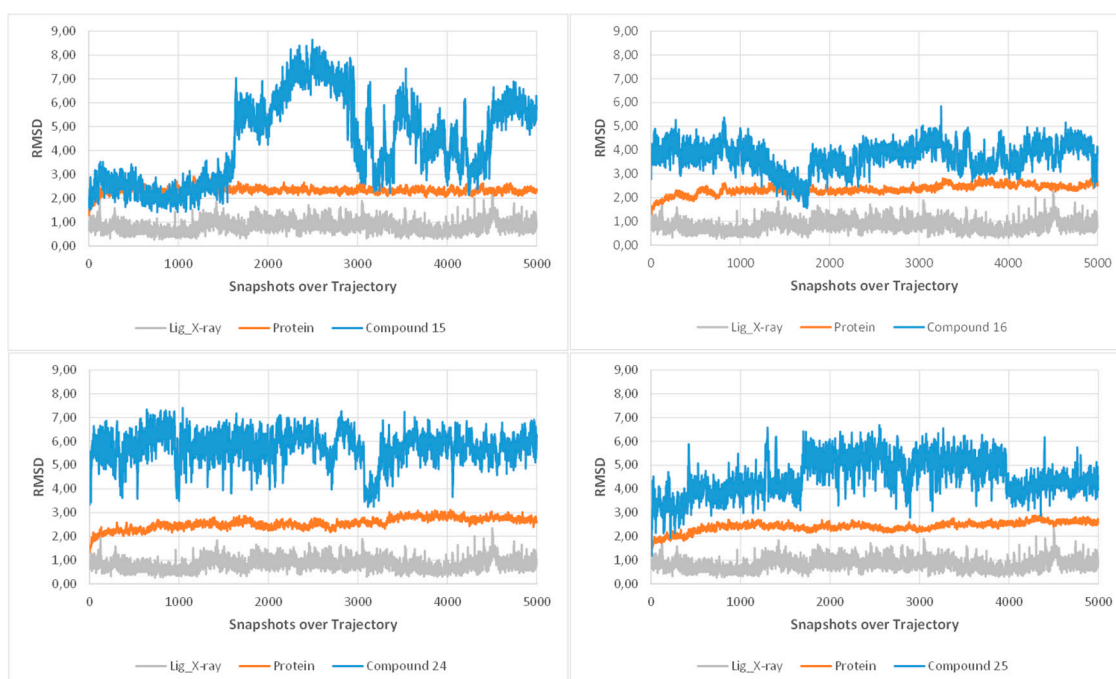
Figure 6. RMSD diagrams from the molecular dynamics simulations for each considered compound (15, 16, 24 and 25). The RMSD values over the trajectory are displayed in orange for the protein and in blue for the ligand. The RMSD values of the reference ligand from 4DXD structure are also displayed for information (data from an independent simulation).
