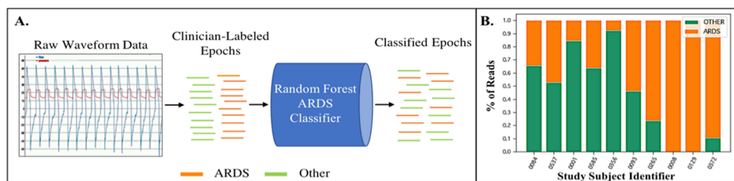
Figure 3. A. Raw waveform data from each 400-breath “read” length is extracted from the ventilator and then attributed as either belonging to an ARDS patient or a non-ARDS patient based on dual clinician diagnosis. These data are then sent to a Random Forest classifier for training. B. Test subjects are then evaluated with the trained classifier. A final diagnosis is performed by the classifier by evaluating which diagnosis received a majority of votes across all reads evaluated by the model in a given period of analysis.
