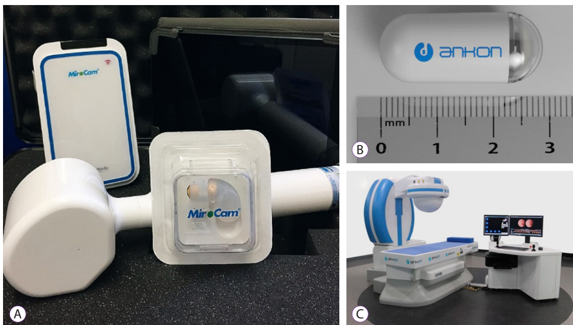
Fig. 1. Magnetically guided (assisted) capsule endoscope. (A) MiroCam NAVI system (Intromedic Co., Ltd., Seoul, Korea). (B, C) NaviCam capsule endoscope and NaviCam magnetic control system (Ankon Technologies Co., Ltd., Wuhan, China).
