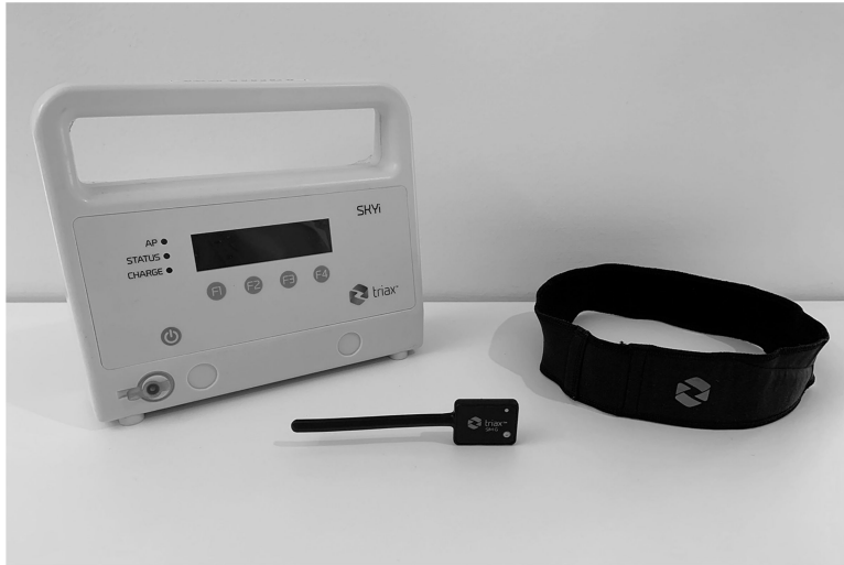
Figure 1. SIM-G impact sensor device (center), neoprene headband (right), and SKYi box (left).
