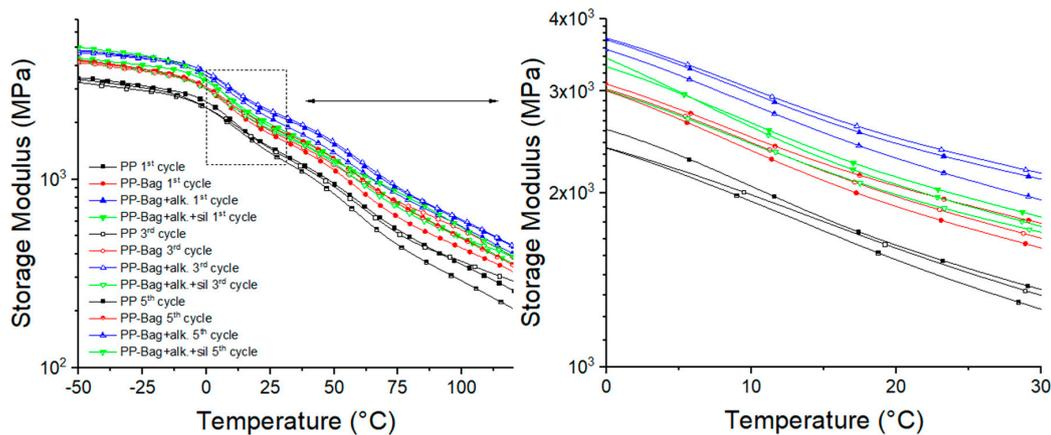
Figure 13. Temperature dependence of the storage modulus of PP and their biocomposites.
