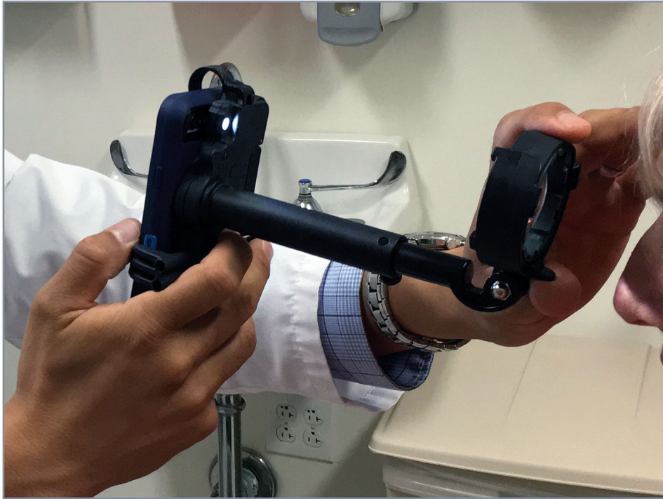
Figure 1. Photograph of the Paxos Scope smartphone adapter. An indirect ophthalmoscopy lens was fitted to the adapter, which together were coupled and aligned to the camera lens of an iPhone.
