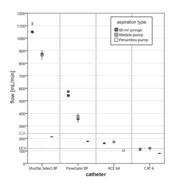
**FIG 1.** Flow through an 8F long sheath (Shuttle Select), an 8F balloon-catheter (FlowGate<sup>2</sup> Balloon Guide Catheter), an ACE 64 distal aspiration catheter, and an AXS Catalyst 6 Distal Access Catheter. Left, Syringe; middle, Medela pump; right, Penumbra pump. *Dark gray horizontal lines* mark the blood flow in the internal carotid artery and the middle cerebral artery in an average patient.
