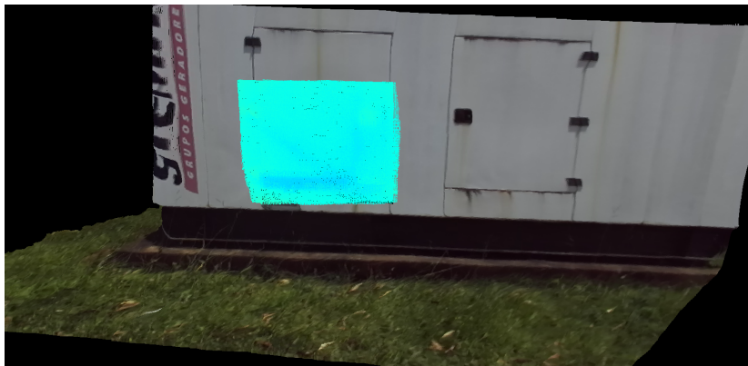
Figure 15. Temperature correction in the 3D model due to a reading from another angle.
