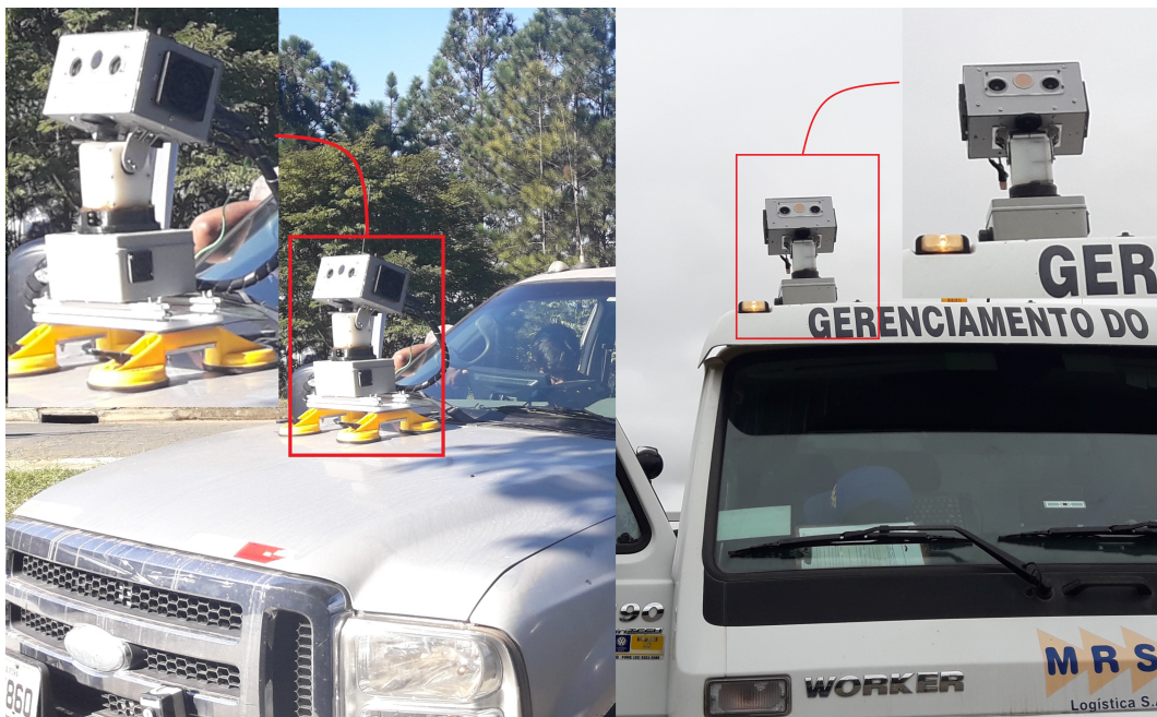
Figure 8. Robot assemble in two different configurations and inspection vehicles.
