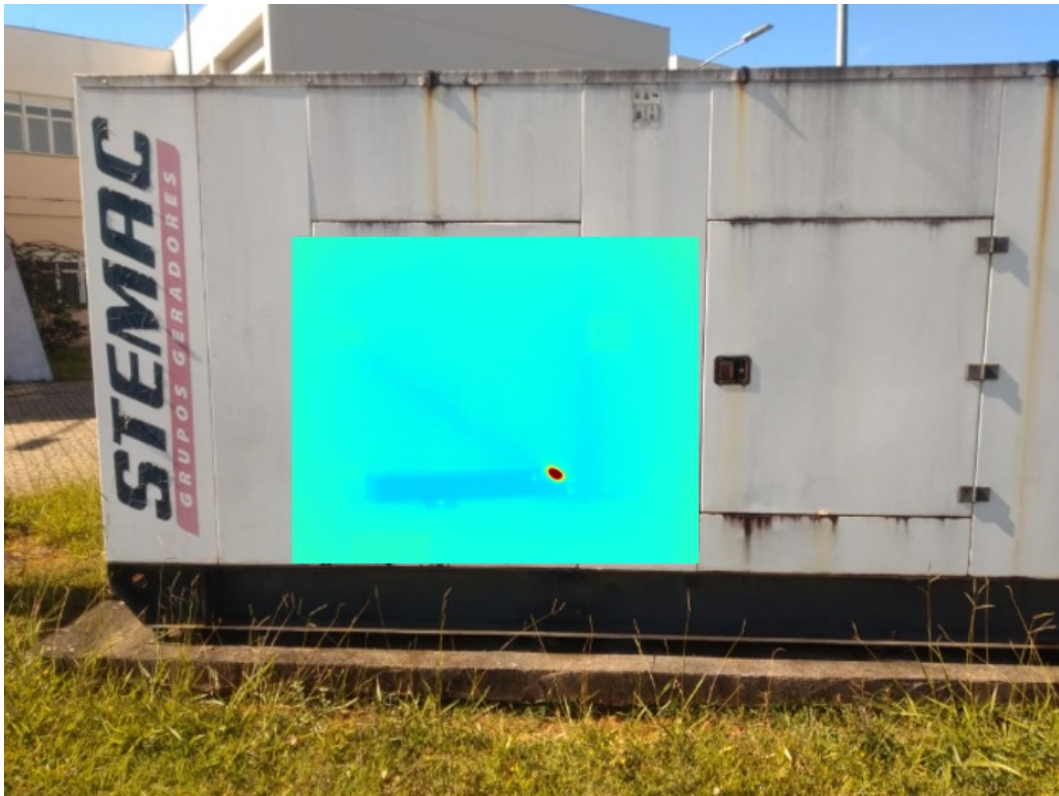
Figure 2. Thermal and Visual homography transformation result.
