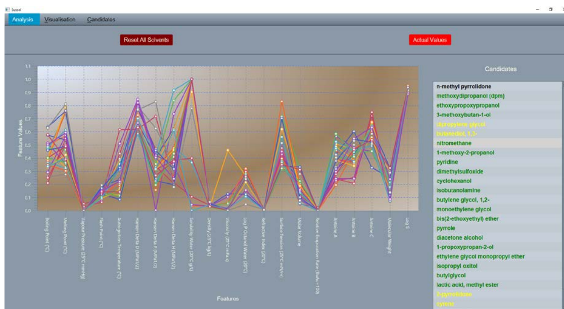
Figure 11. Visualization of candidates list in SUSSOL software. View can be switched between normalized and actual values. The candidate list in the screenshot is not complete. In the software, the scroll bar can be used to view the complete list. Protic solvents are still present in the list in the screenshot.
