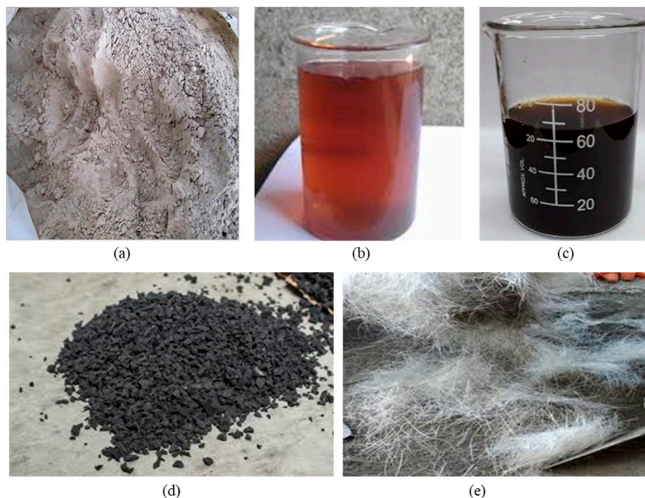
Figure 1. Materials used: (a) class F fly ash; (b) superplasticizer (Sika Viscocrete-2044); (c) graphene oxide; (d) crumb rubber; and (e) PVA.
