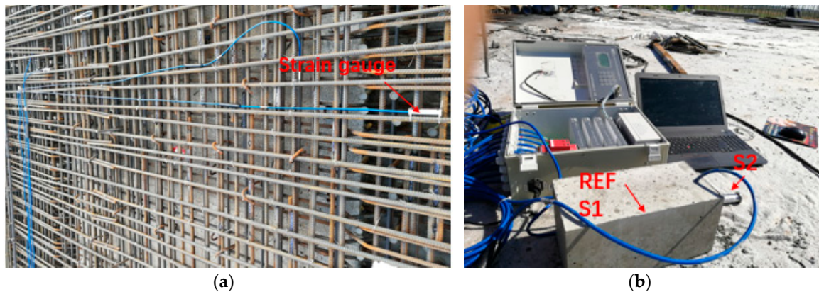
Figure 3. Field arrangement of strain gauge: (a) placement of strain gauge; (b) data acquisition. Where strain gauge 1 (S1) was used to measure the temperature and deformation of Ref, and S2 was used to measure the surface temperature of the deck.
