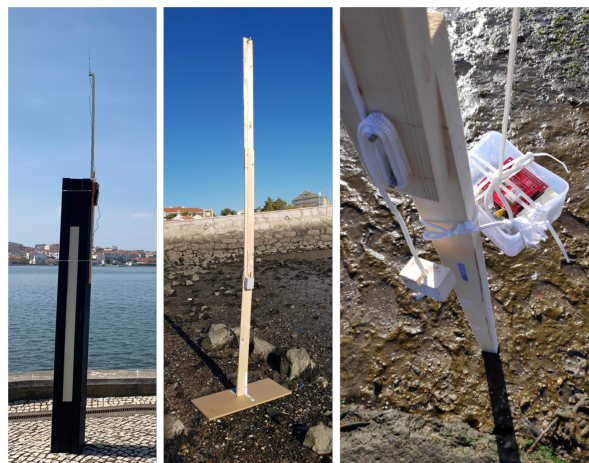
Figure 6. Gateway and sensor nodes in the monitoring field.
