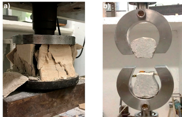
Figure 3. Plain foamed concrete (PFC) specimens: (a) after the compression test and (b) after the tension test.
