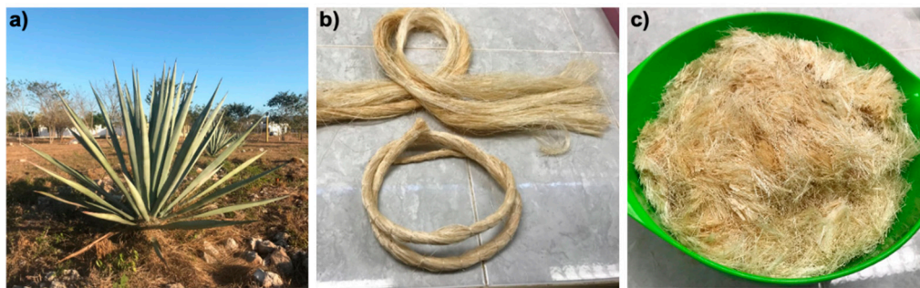
Figure 1. (a) Henequen plant; (b) henequen fibers and (c) henequen fibers chopped to a length of 19 mm.
