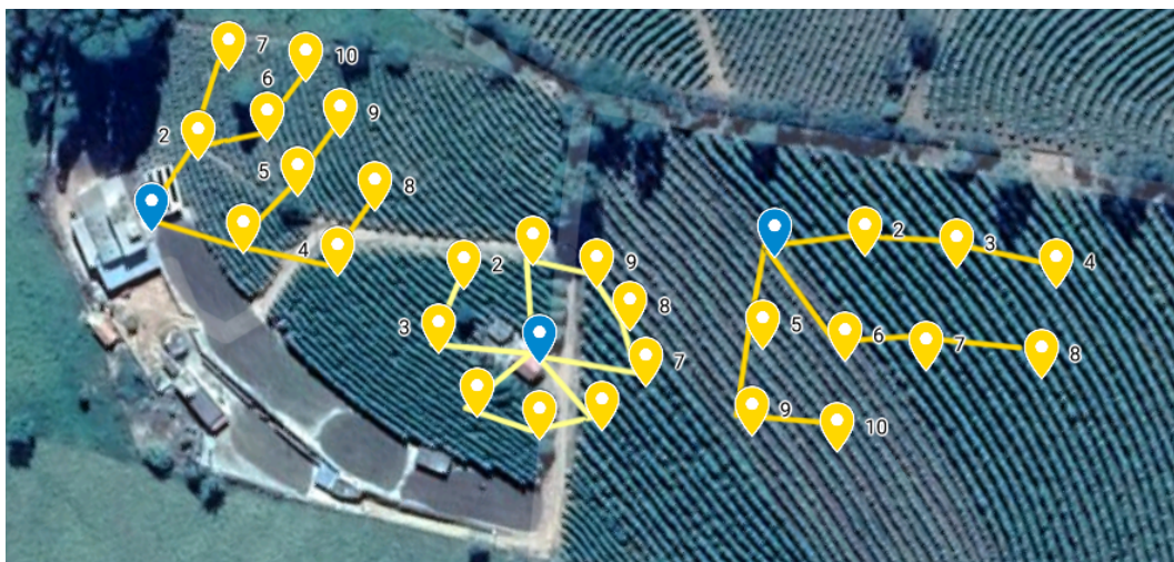
Figure 1. A real monitoring scenario for a coffee plantation with three different topologies, which are tree, circular, and grid topologies.
