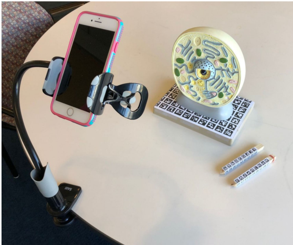
Fig. 1. CamIO system overview. A 3D biological plant cell model is mounted on the CamIO board barcode pattern. The reading and writing styluses (the writing stylus has a red rubber band on its end) are next to it. The CamIO app is running on the iPhone 8, held by a gooseneck cell phone holder clamped to the table, with its main camera aimed towards the cell model.
