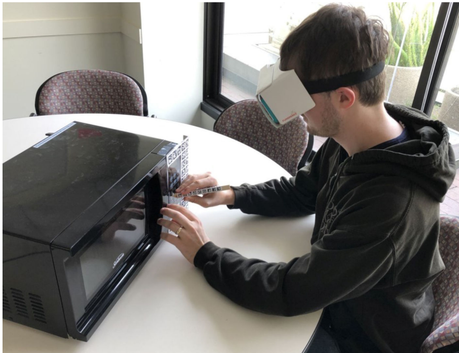
Fig. 3. Study participant using CamIO with Google Cardboard, worn hands-free with a head strap, to access the microwave oven. Participant uses audio feedback from the CamIO app to help aim his head towards the microwave oven panel.
