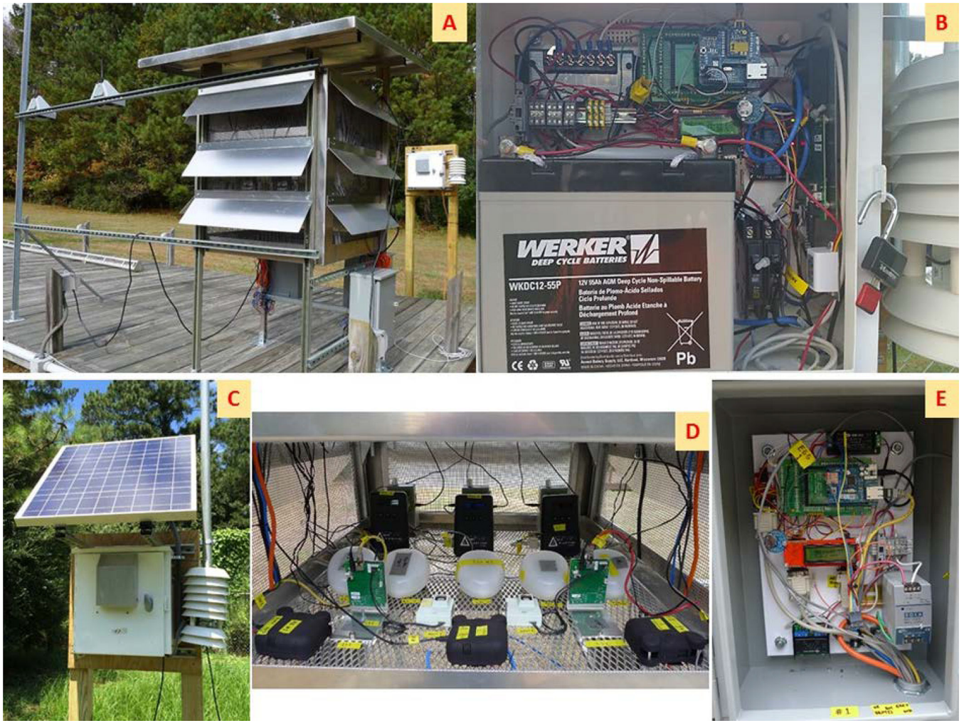
Figure 1. CAIRSENSE field equipment, including (A) SAFT instrument enclosure, (B and C) solar-powered WSN node, (D) interior of SAFT instrument shelter, and (E) WSN node utilizing 120 V (nominal) AC electricity.
