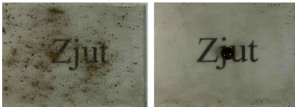
Fig. 22. Spread dust particles (left) and self-cleaned superhydrophobic coating (right)(102). Reproduced with permission from Elsevier.
