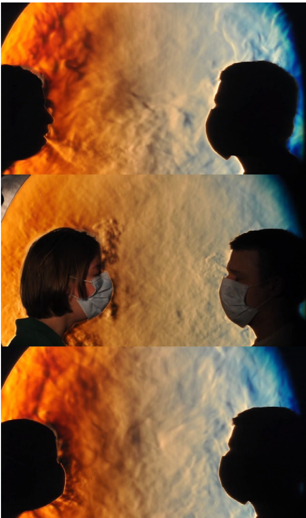
Fig. 22 Schlieren images of two volunteers. The roughness of the Schlieren image is related to the turbulence of the emission, and visualizes the fluid flow of the emitted aerosols. In one instance, a person coughs without any mask protection (top), wearing a surgical mask (middle) and finally a FFP2 mask (bottom). The flow direction is inclined 308^\circ downward in the top image. It has both vertical components (downward and upward) and lateral components that bypass the surgical mask in the middle image. The best fit of a FFP2 mask reduces the bypass flow but it increases the flux released through the mask. However, its weak speed limits the region affected by exhalations to the immediate neighborhood of the volunteer (images provided by Gary S. Settles)
