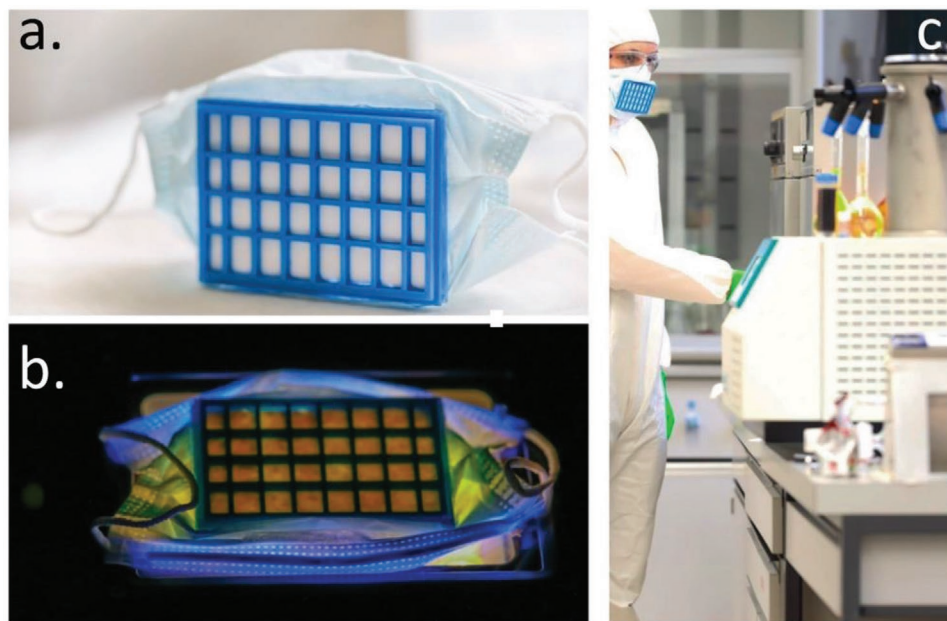
Figure 6. The reusable protective mask designed around the \text{TiO}_2\text{NWs} -based filter paper. a) Photo of the mask prototype in which the \text{TiO}_2\text{NWs} filter paper is attached to a 3D-printed plastic frame. b) Photo of the mask prototype during its disinfection under 365 nm UV illumination. The filtered germs are inactivated by ROS, formed in the photocatalytic reaction on the surface of the filter material. c) Photo of the reusable protective mask prototype in real conditions (courtesy of Swoxid S.A.).
