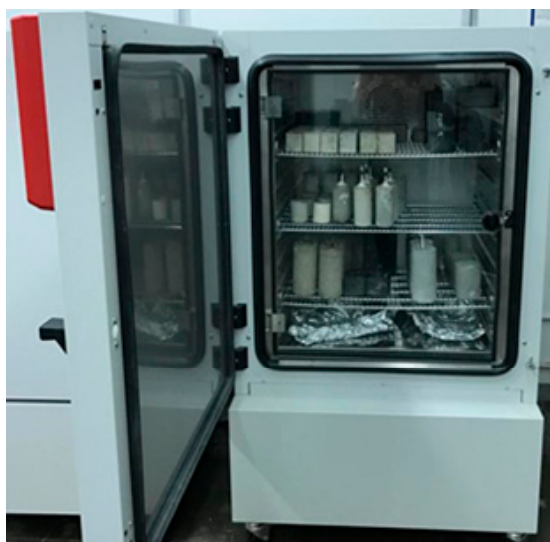
Figure 12. Climate chamber for the CO 2 exposure under the controlled conditions.
