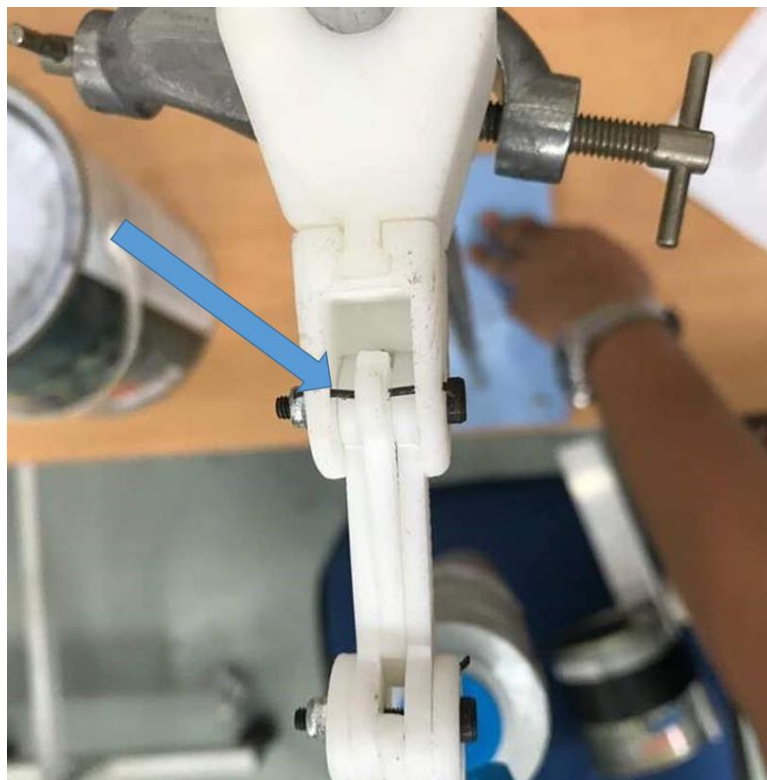
Figure 21. Bending effect of the pin (A) of JCC at maximum load for ABS structure.
