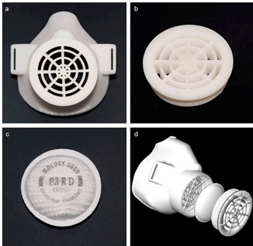
Figure 9. Custom made 3D protective face mask. (a) Reusable 3D-printed face mask, (b) filter membrane support, (c) filter membrane and (d) 3D image of the prototype.
