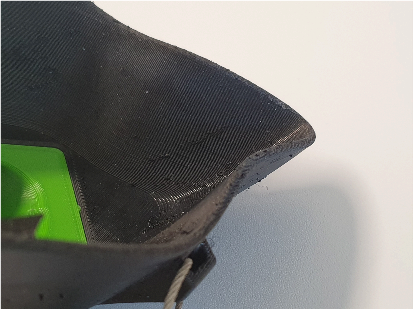
Fig 6. Edge of the printed mask. The edge of the printed mask is made of the same material as the mask itself and therefore relatively thin.
