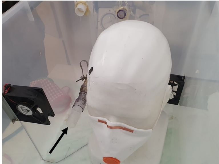
Fig 3. Measuring box. Photo from inside of the measuring box with the open pipe (arrow) and the mask attached to the phantom head.
