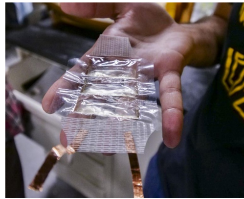
Fig. 3 A view of the hydraulically amplified self-healing electrostatic actuator [129]
