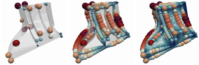
Fig. 7. The three phases of VoroCrust refinement demonstrated on the Fandisk model: protection by corner balls (left) followed by edge balls (center), and finally coverage by surface balls (right).
