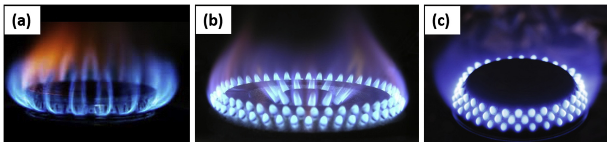
Fig. 8 – Comparison of (a) natural gas, (b) H_2 enriched natural gas, and (c) H_2 flames for thermal energy applications.
