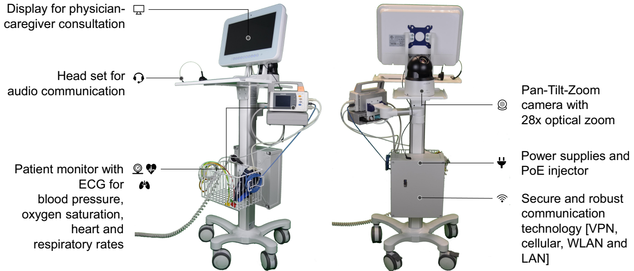
Figure 3 The TeleDoc version 1 prototype consist of two sides. The front side equips software and hardware components required by the nurse. A Pan-Tilt-Zoom camera is provided at the back side and is directed towards the patient.
