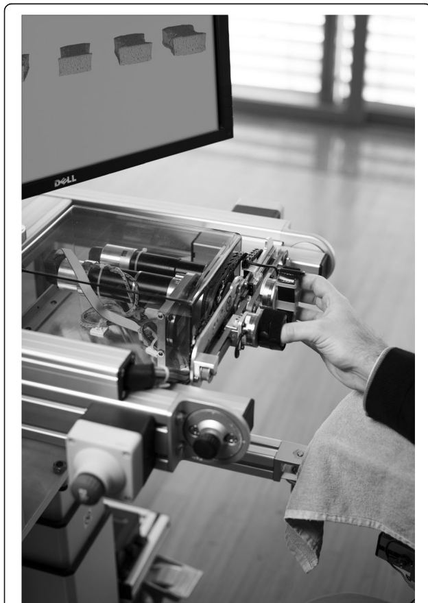
Fig. 1 A subject with stroke using the ReHapticKnob. The ReHapticKnob is a haptic device used to train hand opening-closing and forearm pronosupination. The device integrates a set of 7 therapy exercises reproducing typical neurocognitive exercises [29]. In the present exercise, the compliance of different virtual sponges rendered by the device has to be memorized and identified by relying on hand somatosensory inputs during active interaction with the device
