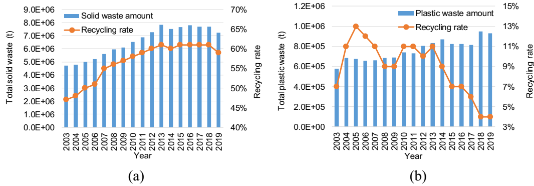
Fig. 3. Waste generation and its recycling rate from 2003 to 2019 in Singapore. (a) Total solid waste and overall recycling rate; (b) total plastic waste and plastic recycling rate. Data from NEA (2020a).
