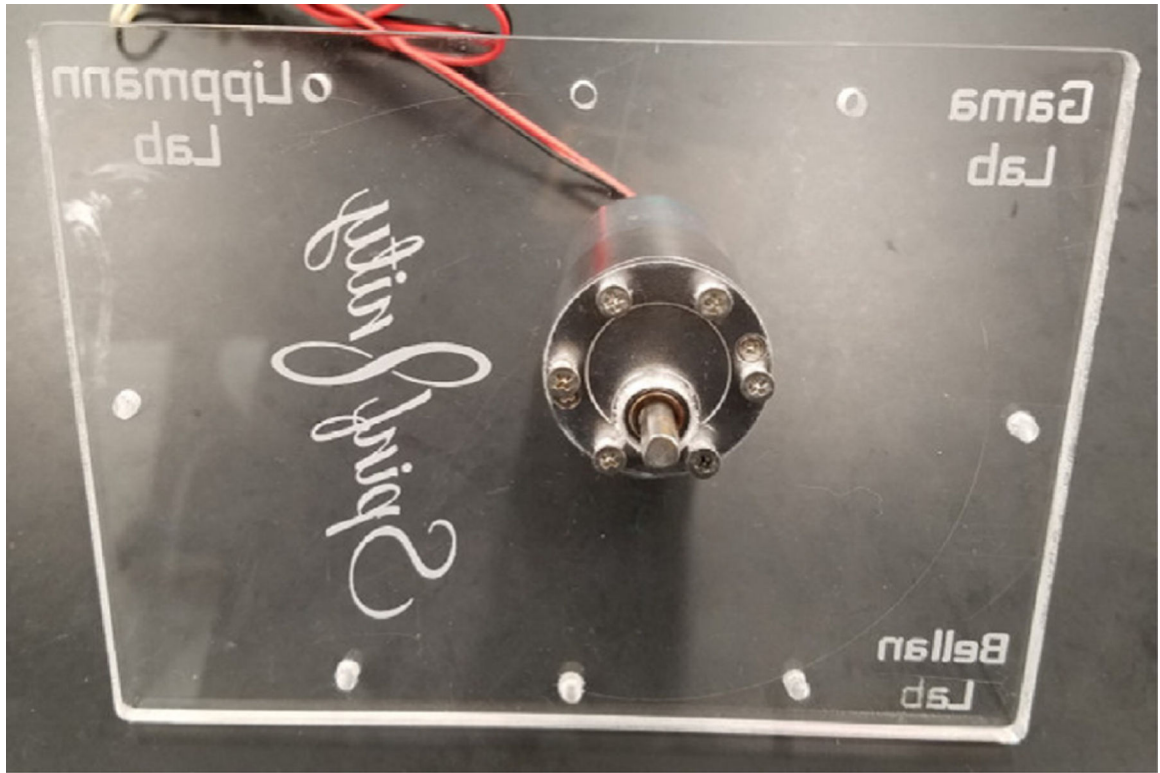
Fig. 10. Attachment of the motor to the acrylic plate.
