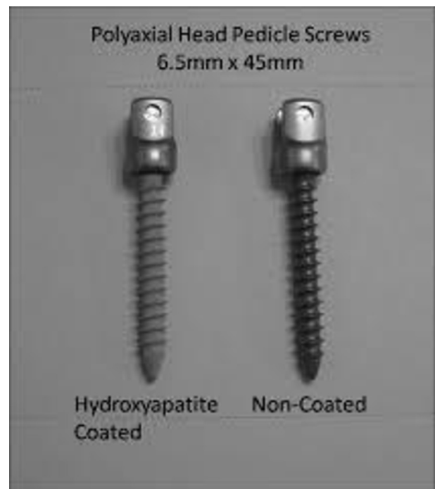
Fig. 8. 43 Image showing a HA coated screw and a traditional screw.
