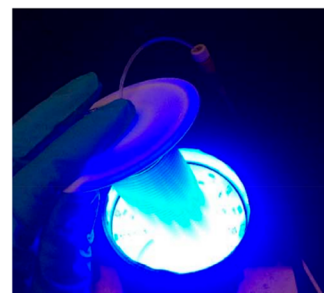
Figure 26. (A, B) Photocatalytic alkylation reaction in batch versus in stop-flow microtubing reactor. Graphs in panel B are reproduced from ref 102. Copyright 2017 American Chemical Society.
