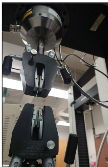
Fig. 25. Mechanical testing of swabs with an Instron 4206.
