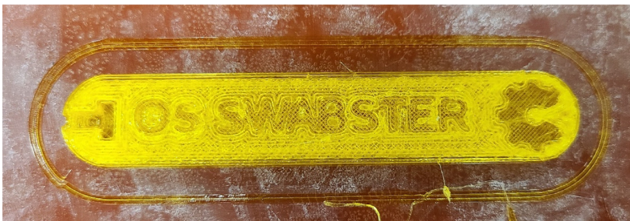
Fig. 21. As printed version of handle on a Lulzbot Taz 6 print bed.
