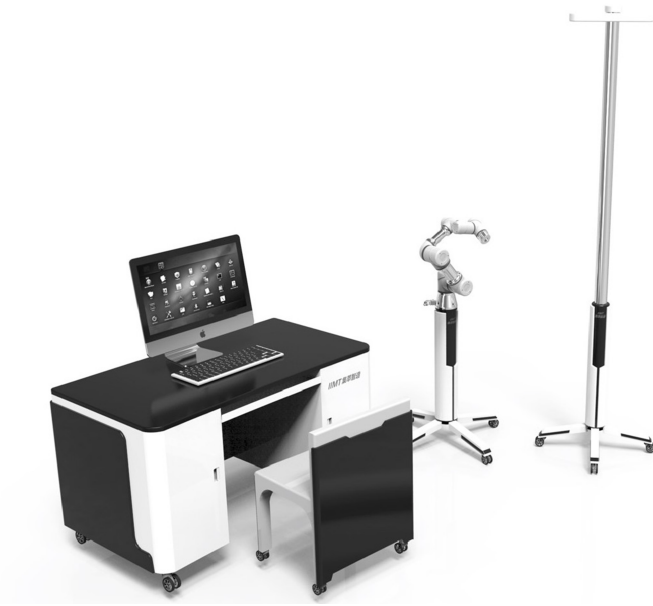
Figure 1 Schematic diagram of the binocular-stereo-vision-based navigation robot. The navigation robot was composed of binocular stereo visual tracking equipment, an operation planning and controlling system and a six-axis robotic arm.
