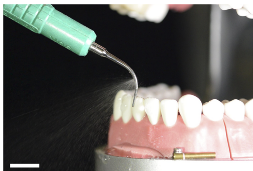
FIG. 3. Image of the Cavitron scaler adjacent to a dental mannequin installed in a dental chair in the experiments in the dental clinic. Still image taken from video 3, water being the working fluid. Scale bar: 1 cm. Multimedia view: https://doi.org/10.1063/5.0021476.2
