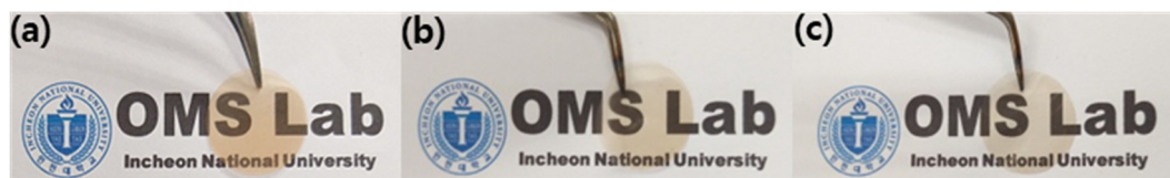
Figure 2. Photographs of the synthesized polymer membranes (a) x(10:0.75:0.25) ; (b) x(10:0.5:0.5) ; and (c) x(10:0:1) .
