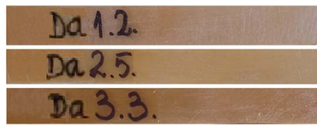
Figure 1. Hybrid resin sample with a volume ratio of 60% (Da 1.2), 70% (Da 2.5), and 80% Dammar (Da 3.3) respectively.
