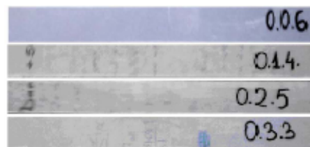
Figure 2. Samples of composite materials reinforced by waste paper sheets, with an epoxy resin matrix (0.0.6) and, respectively, hybrid resin with a Dammar volume ratio of 60% (0.1.4), 70% (0.2.5) and 80% (0.3.3).
