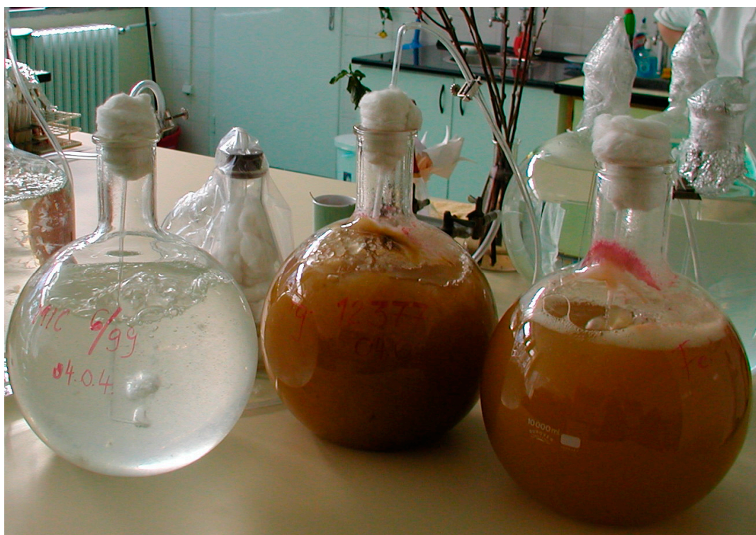
Figure 12. Bubble-breeding (BB) method for inoculum production. Left: A young inoculum 2–3 days old, right: Ready inocula for use before terminating the breeding.
