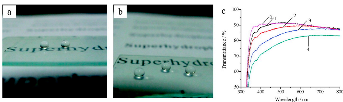
Figure 6. Digital photos of glass slides with superhydrophobic coatings prepared by dip-coating the APTS-modified HSPs: (a) APTS 0.70 wt % and (b) APTS 0.90 wt %. (c) Transmission spectra of coatings on glass slides: (0) bare glass slide and (1–4) slides prepared by dip-coating the 0.30 wt %, 0.50 wt %, 0.70 wt %, and 0.90 wt % APTS sols. Adapted with permission from [107]. Copyright (2012) American Chemical Society.
