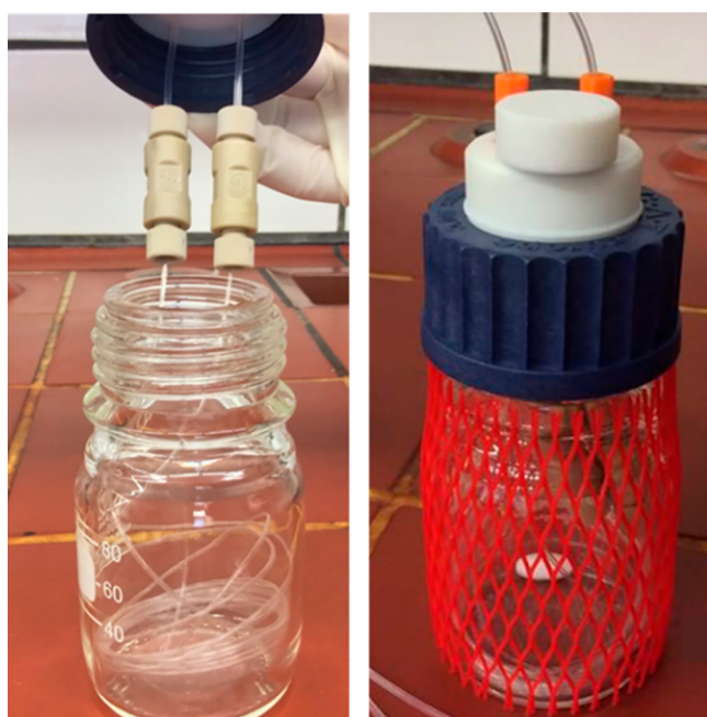
Figure 4. Tube-in-flask setup with the AF-2400 membrane coiled inside a standard flask.
