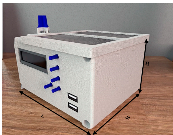
Figure 11. Proposed prototype for measurement of sunshine duration (SD).
