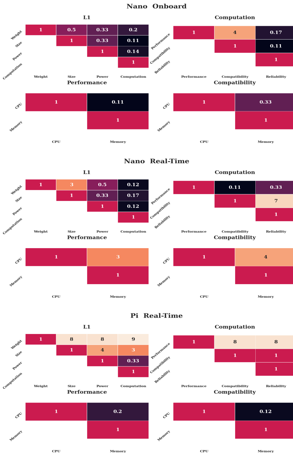
Figure 11. The weight matrices leading to the highest preferences for each alternative . The first heat maps show the weights for the Nano-onboard- alternative , the second set of heatmaps the weights for the Nano-real-time- alternative , and the third row the weights for the Pi-real-time alternative . The top row shows the first two levels, the bottom row the third level. Only the upper diagonal weights are shown for simplicity. Darker colors indicate less preference, lighter colors more preference.
