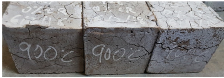
Figure 5. CR-ECC with 0% CR at 900 °C.
