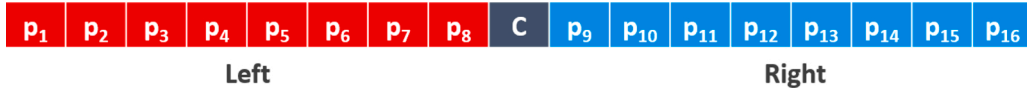
Fig. 1. The used 17 sized windows. The 9th value of this window assigned as center value and contamination area of it is shown. The contamination area is categorized into two groups, and these groups are called left and right.
