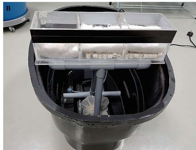
Figure 5. Trickle box filter system. (A) Assembled using 5 mm transparent acrylic sheet, the trickle box is placed on the water reservoir to collect water from the drainage line and filter it before returning the water to the water reservoir. Each compartment contains ceramic rings and cotton sponge filter. Arrows shows the flow of water. (B) The trickle box filter system is placed on the water reservoir by sitting on a holder made with PVC fittings.
