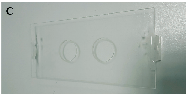
Figure 3. Zebrafish tank with lid. (A) Each zebrafish tank is made of 5 mm transparent acrylic sheet, gluing with marine-safe acrylic glue. Each can hold 6 L water, making each tank could house a total of 30 zebrafish (5 fish/L). The outlet of the tank is constructed by drilling a hole on one side of the tank, and fix with a PVC fitting V-tank connector and an equal elbow. A mesh is installed onto the outlet, preventing fish from reaching the drainage line. (B) Each tank received continuous flow of water from the supply line. Excess water will then flow into the drainage line through the outlet. (C) The tank lid contains 2 openings used for feeding and as water inlet.
