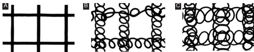
Figure 4. Effect of the applied voltage on the deposited fiber patterns (65 wt/v% polycaprolactone, stage speed = 150 mm/s, D = 3 mm). (A) 2.6–3 kV. (B) 3.2 kV. (C) 3.4 kV
