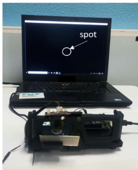
Figure 6. The Cyclops prototype in the foreground, with the camera mounted on the eyewear and connected to a PC in the background (we can notice the white spot). See Video S1.
