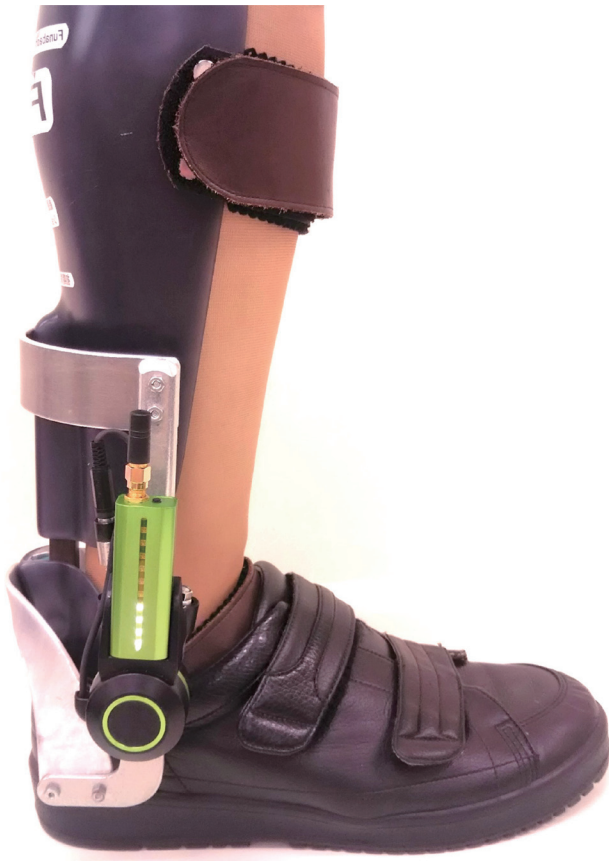
Fig. 2. USB accelerometer and potentiometer affixed to the main body of the AFO-PR using a mounting jig.
