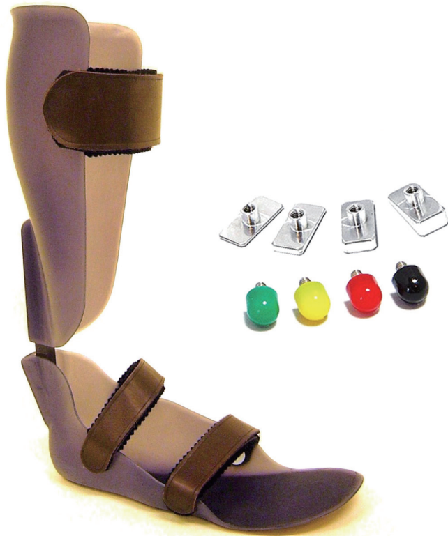
Fig. 1. Appearance of the AFO-PR and the parts used for adjusting the initial dorsiflexion angle and plantarflexion resistance. The initial dorsiflexion angle of the orthosis can be set to 0°, 3°, 6°, or 9° by changing the duralumin spacers, which come in four different thicknesses. The plantarflexion resistance force can be set to 0.5, 1.0, 1.5, or 2.0 Nm/degree by changing the urethane rubber parts, which come in four different levels of hardness.
