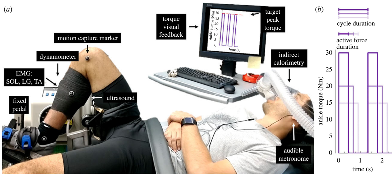
Figure 2. (a) Experimental setup of a participant cyclically generating soleus muscle-tendon force to produce a plantar flexor moment that exerts an external torque on a fixed dynamometer pedal following the cues of an audible metronome and visual feedback. EMG, electromyography; SOL, soleus; LG, lateral gastrocnemius; TA, tibialis anterior. (b) Ankle torque versus time for three conceptual trials that yield the same average ankle torque. (Online version in colour.)
